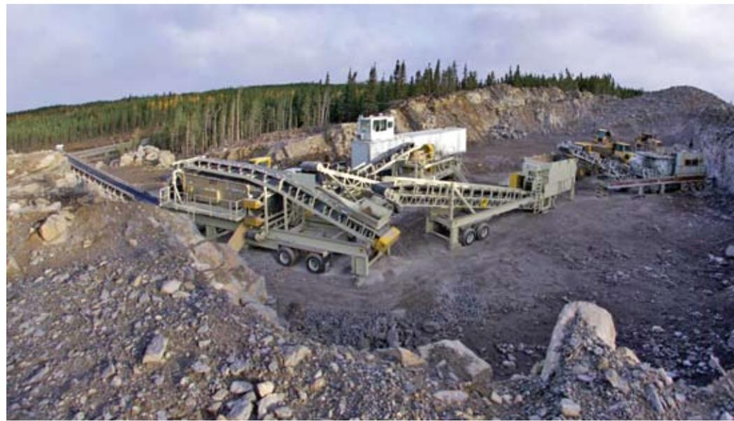
*Rock crusher in quarry preparing granular material for finished grade of access road.*
